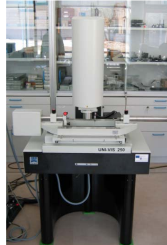
Fig. 8. Deployed multisensor CMM.
