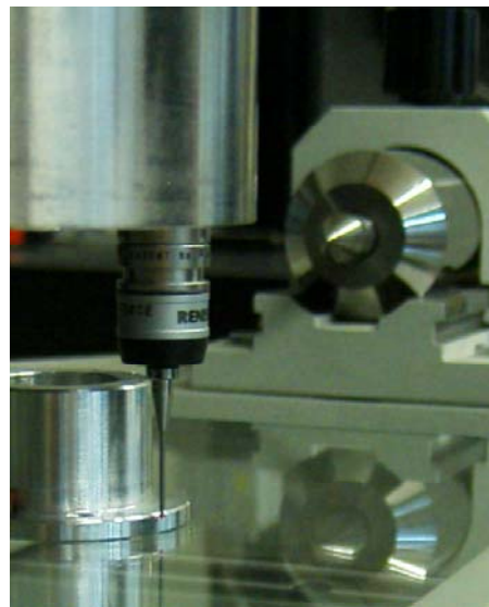
Fig. 9. Measuring object (left part) during the tactile measurement on the CMM.
